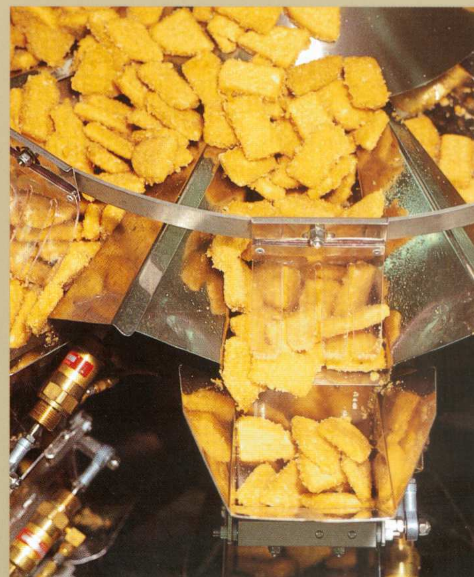
A computer-controlled scale fills each carton to within 3 grams of designated package weight.
